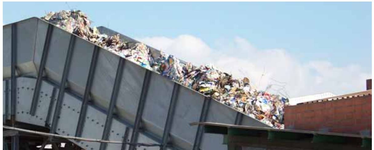
2 The conveyor feeds the cartons into the pulper
